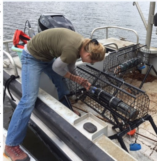
Pictured above: Natural Resource Biologist prepares an automated water quality meter for deployment into Deep Creek Lake
