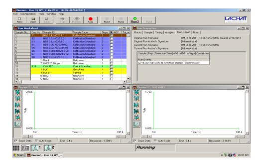
9.2.10 If the calibration passes, instrument will continue to analyze the samples. If it fails, take appropriate corrective actions and recalibrate before proceeding to analyze samples.
