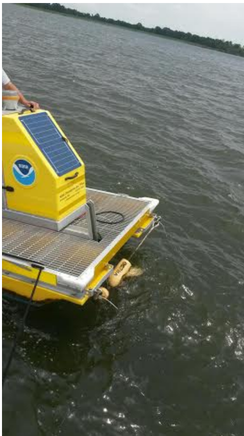
Figure 1. Tangled anchor line.
