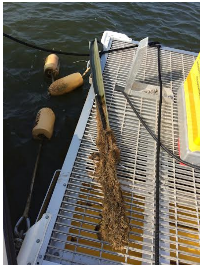
Figure 2. Biofouling on depth sounder.
