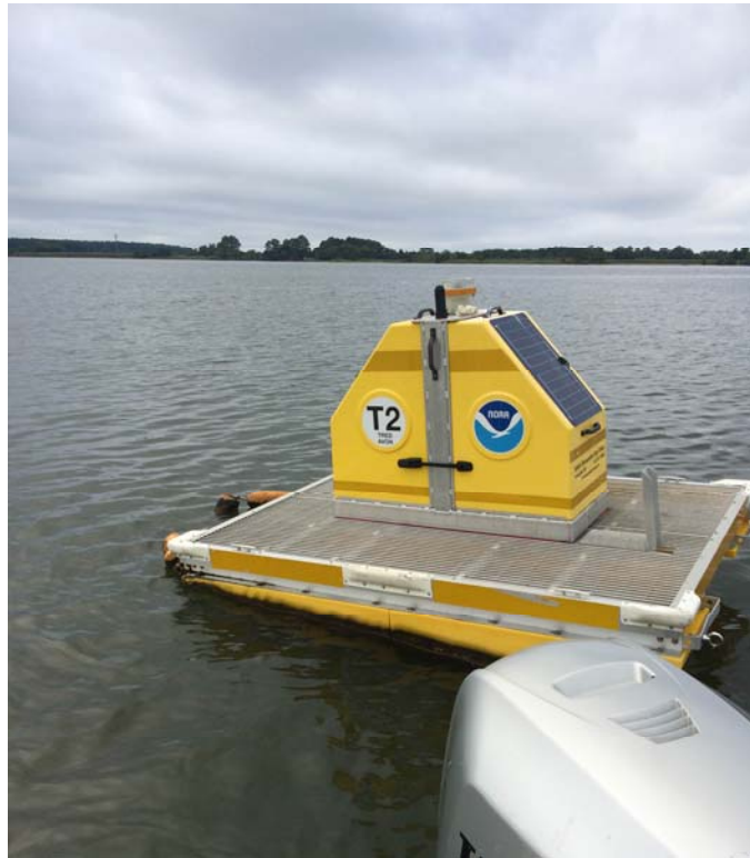
Figure 1. Vertical profiler platform taking on water in one of the platform pontoons (August 16, 2016).
