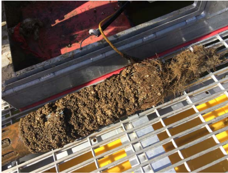
Figure 2. Biofouling on the monitoring sonde at the Tred Avon vertical profiler (August 11, 2016).
