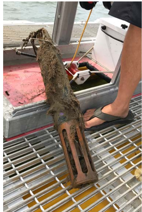
Figure 1. Biofouling on data sonde after an extended deployment at the Tred Avon profiler (July 27, 2017).
