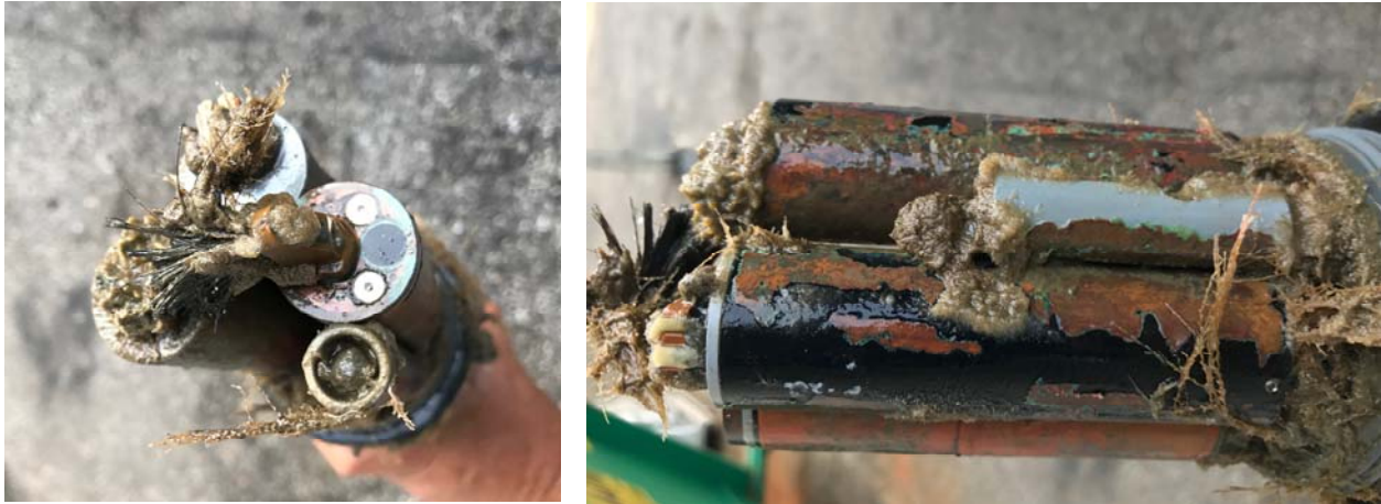
Figure 2(a-b). Biofouling on data sonde after an extended deployment at the Tred Avon profiler (July 27, 2017).
